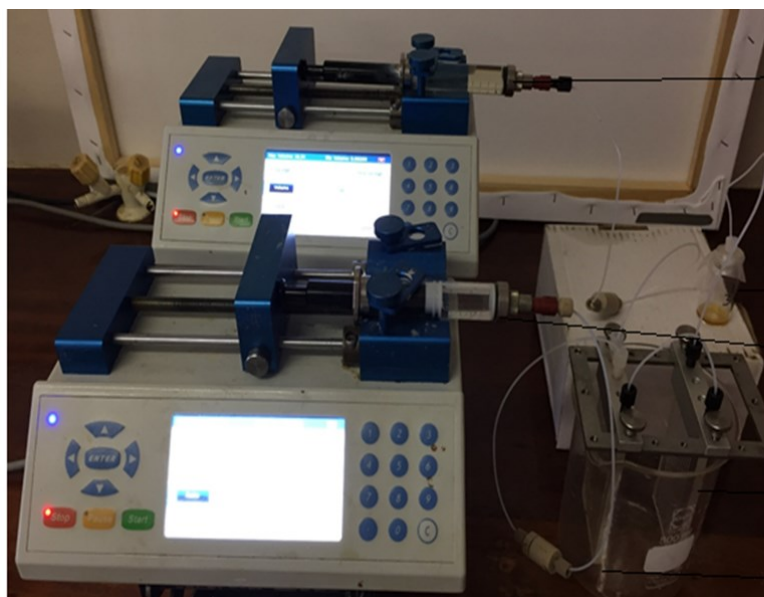
Microreactor set up for flow synthesis of Emtricitabine.
